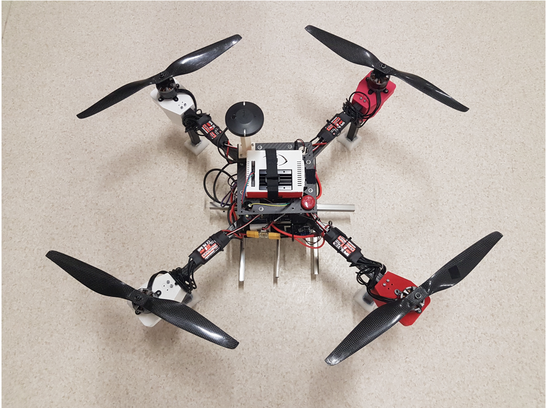
Figure 4.2: A custom-made quadrotor UAV with an RTL-SDR receiver, VHF antenna and on-board computer.
