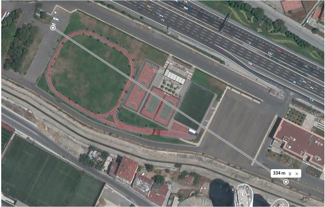
Figure 4.7: Signal sample taken from 30 meters height from ground and 334 meters distance to target. The UAV is in the start of the line, and the target is in the point where distance is shown on. This field is also the area where the experiments are performed.
