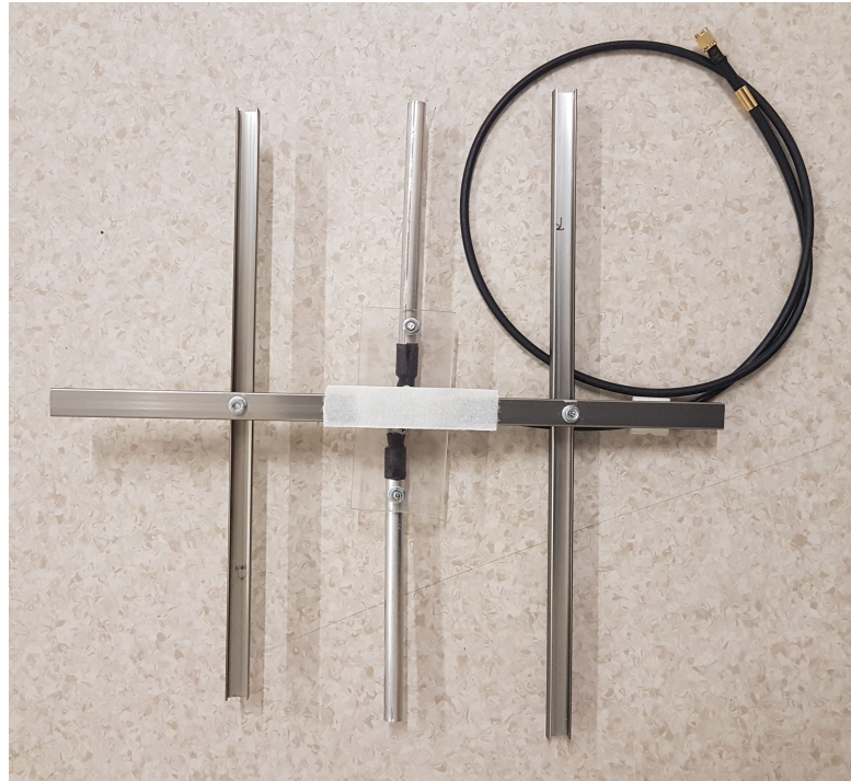
Figure 4.3: 3-Element Yagi-Uda Antenna.
