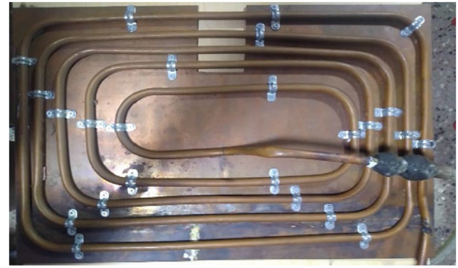
Fig. 2. Pictorial view of a spiral flow thermal collector.
