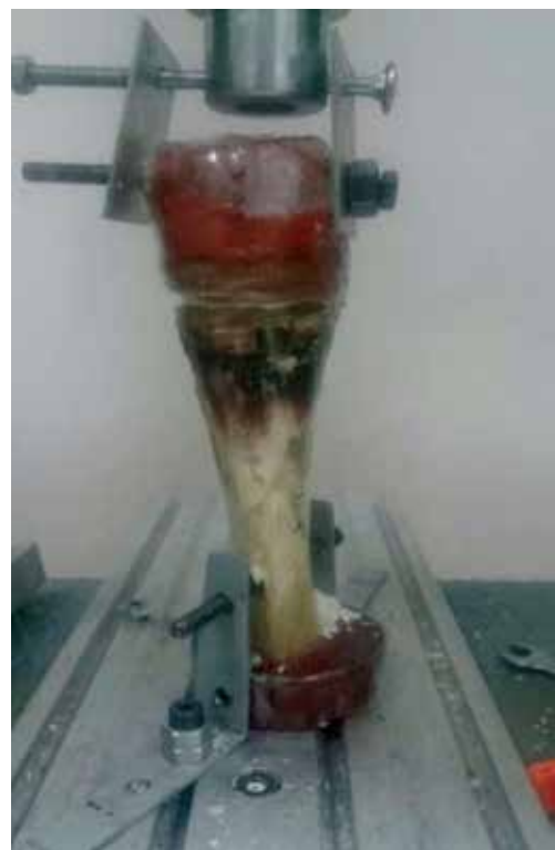
Figure 4. Bicortical screw tensile force application.
