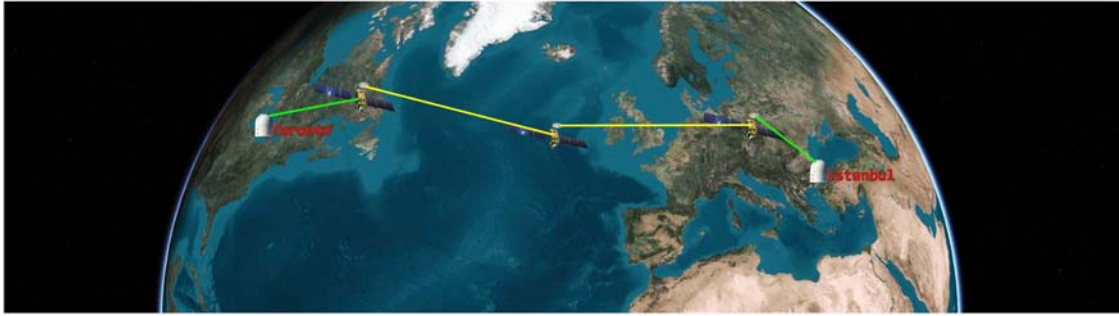
FIGURE 1. Illustration of a shortest path for a longer LISL range for an inter-continental connection from Toronto to Istanbul.
