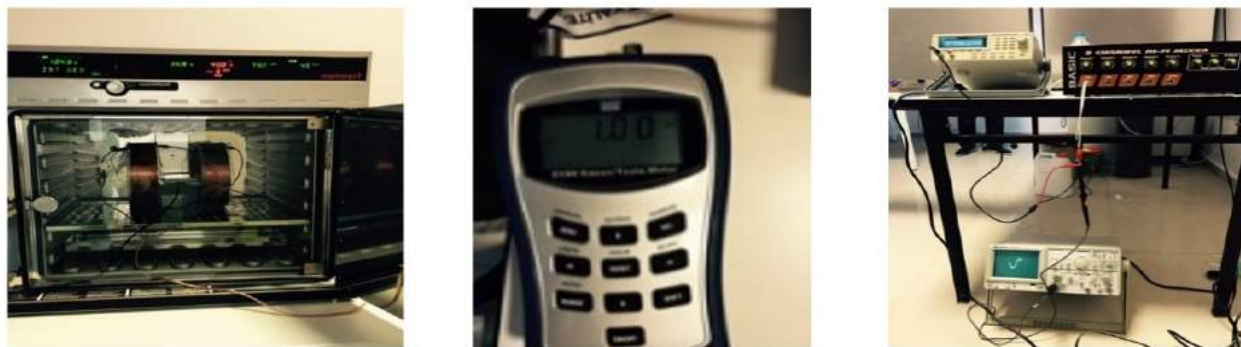
Figure 1. ELF-EMF exposure system
