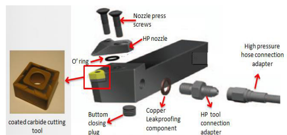
Fig. 3. Coated carbide cutting tool and Jet stream PCLNR tool holder.
