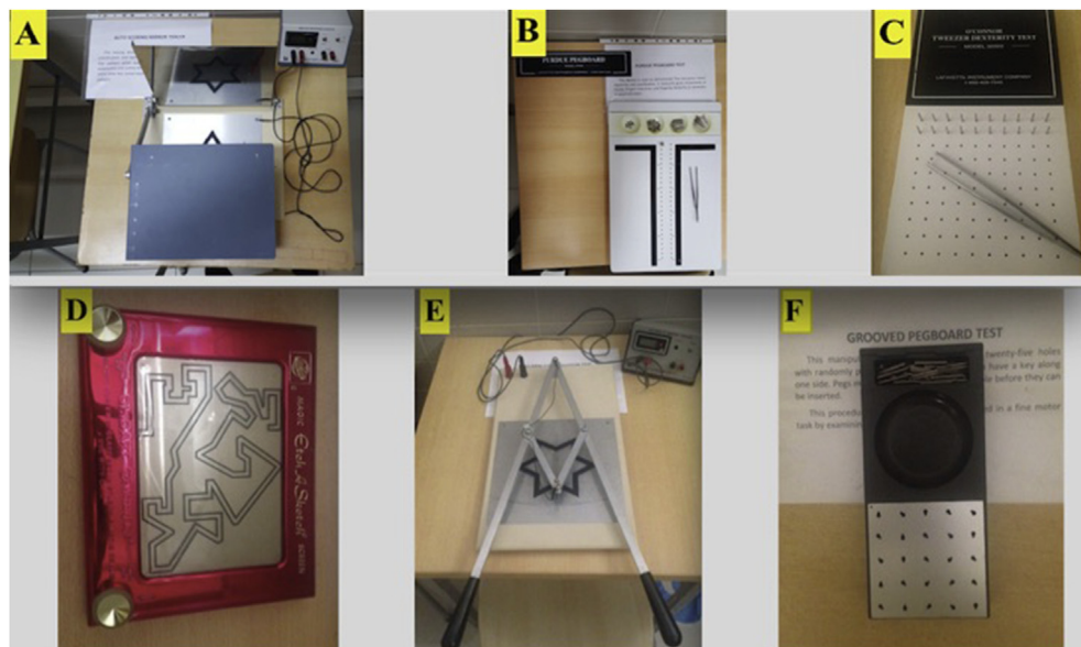
Fig. 1. A) Auto Scoring Mirror Tracer, B) Purdue Pegboard, C) O'Connor Tweezer Dexterity Test, D) Etch-a-Sketch with Overlay, E) Two Arm Coordination Test, F) Grooved Pegboard Test.
