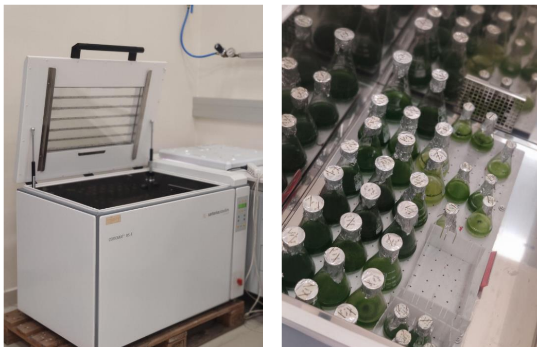
Figure 10. The shaker device used for cultivation
