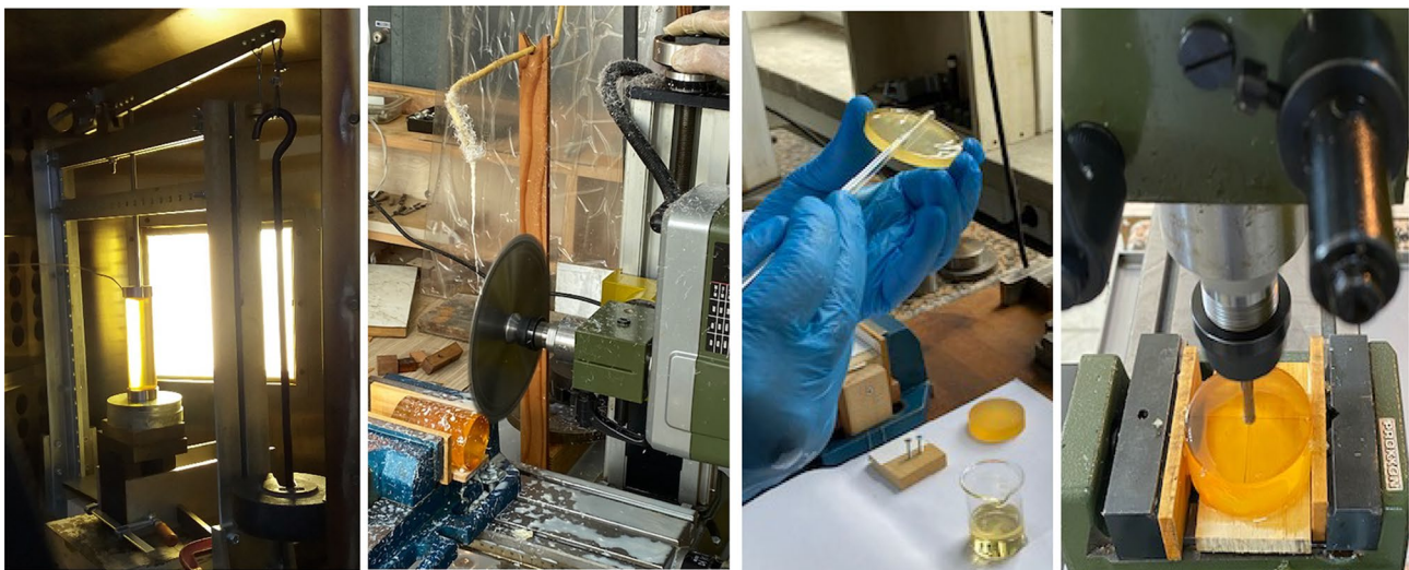
Fig. 2 Some steps of the preparation of the model: The axial loading is applied to a cylindrical Araldite to obtain the mechanical model of the thermal strain in the axisymmetric cross-section of the first layer of the model. The first layer is sliced using a precise cutting machine with cooling lubricant. The layers are bonded to each other applying an epoxy-based adhesive to interfaces. A cavity is drilled with lubricant in the first layer of the model to represent a defect
