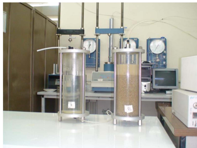
Fig. 1. Bentonite injection in sand test setup. (Image by Mucahit Namli.)
