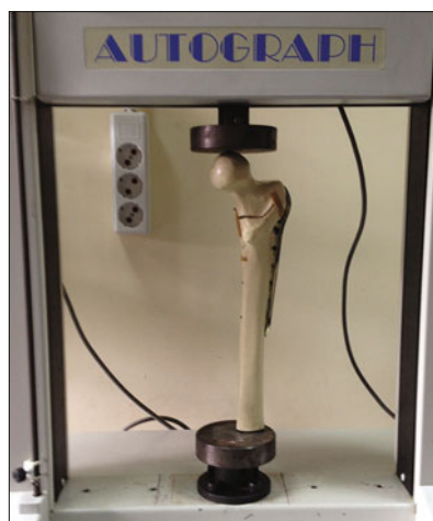
Figure 3: Positioning of bone-implant construct and biomechanical loading test with Shimadzu Autograph AGS testing device
