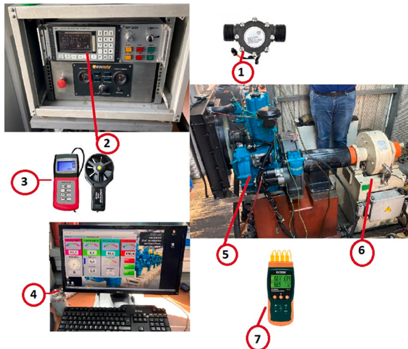
1.) Water Flow Meter 2.) Dyno PID Control Unit 3.) Anemometer 4.) Data Acquisition and data monitoring device 5.) Diesel Test Engine 6.) Eddy-current Dyno 7.) Temperature Measurement Device
