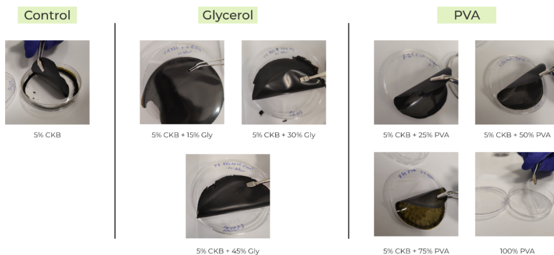
Figure 40: Image of all film groups made directly from Klebsormidium and prepared with PVA and Glycerol additives.
