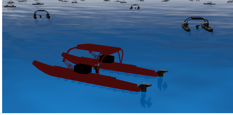
Figure 1.3: Snapshot from the simulation environment populated with 100 vessels. The red USV will be controlled by the motion planning algorithm developed by the user.
