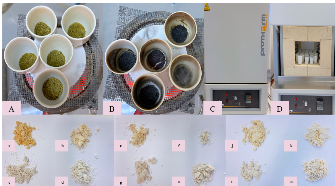
Figure 5. Stages of ash analysis.
