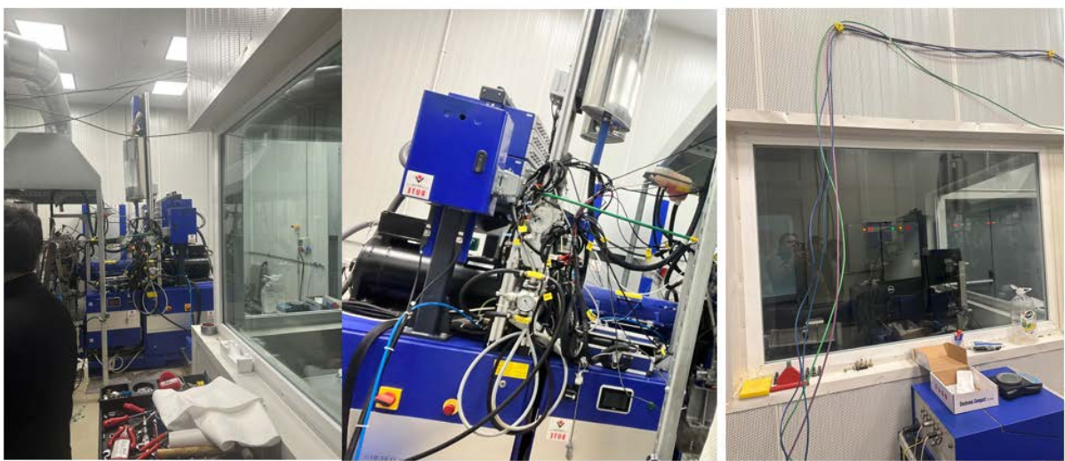
Figure 19. Engine–Dynamometer Laboratory Layout and Control Room Interface
