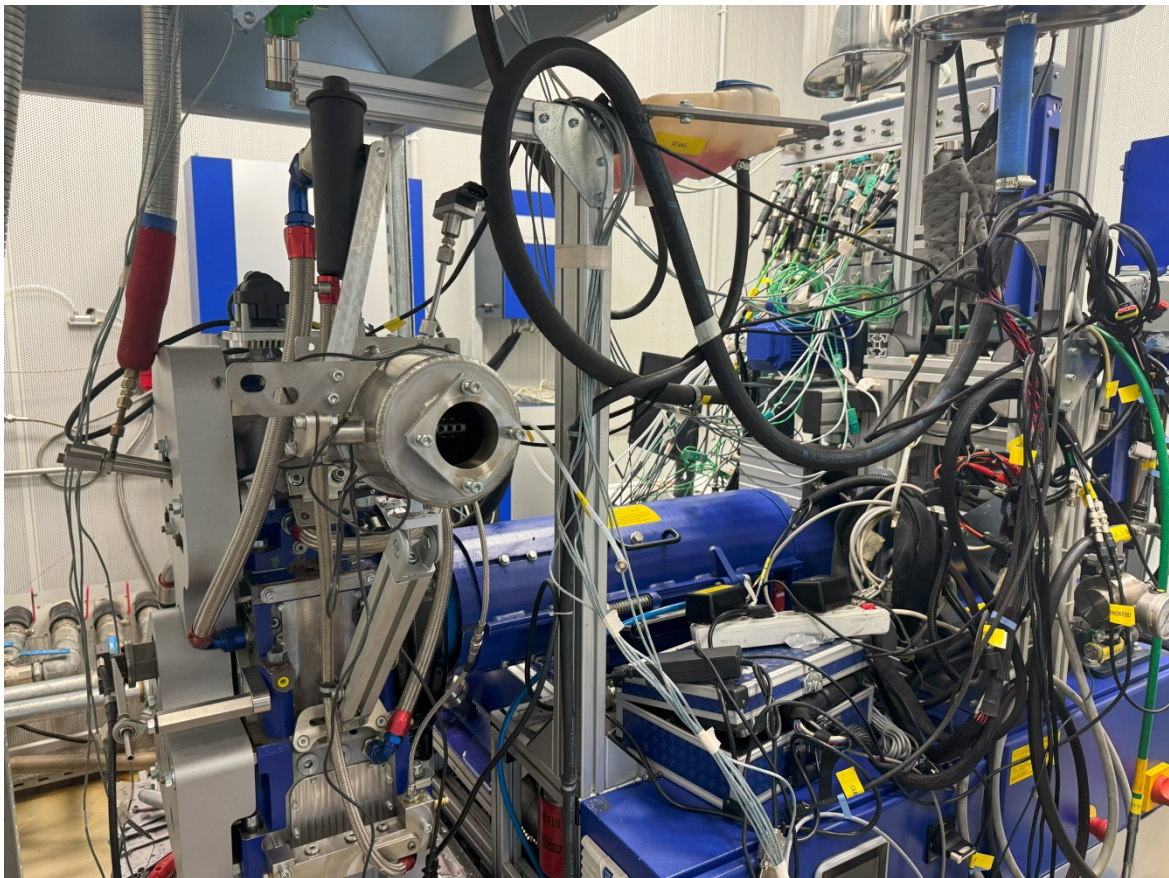
Figure 20. Fully Instrumented Engine–Dynamometer Test Configuration
