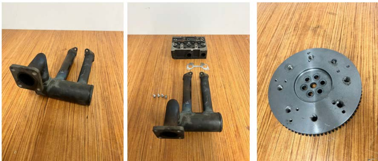
Figure 13. Custom-designed components for engine–dynamometer interface preparation during our engine dynamometer test.
