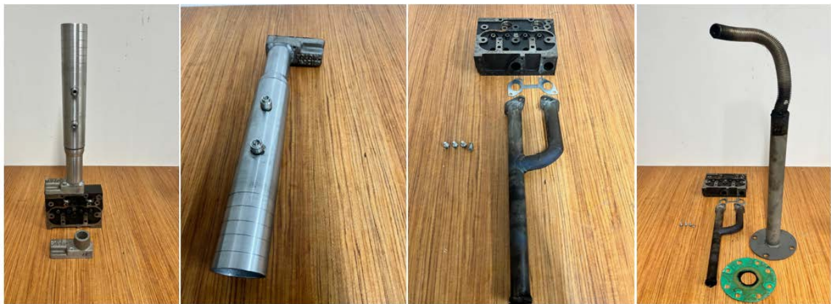
Figure 12. Custom-Designed Components for Engine–Dynamometer Interface Preparation
