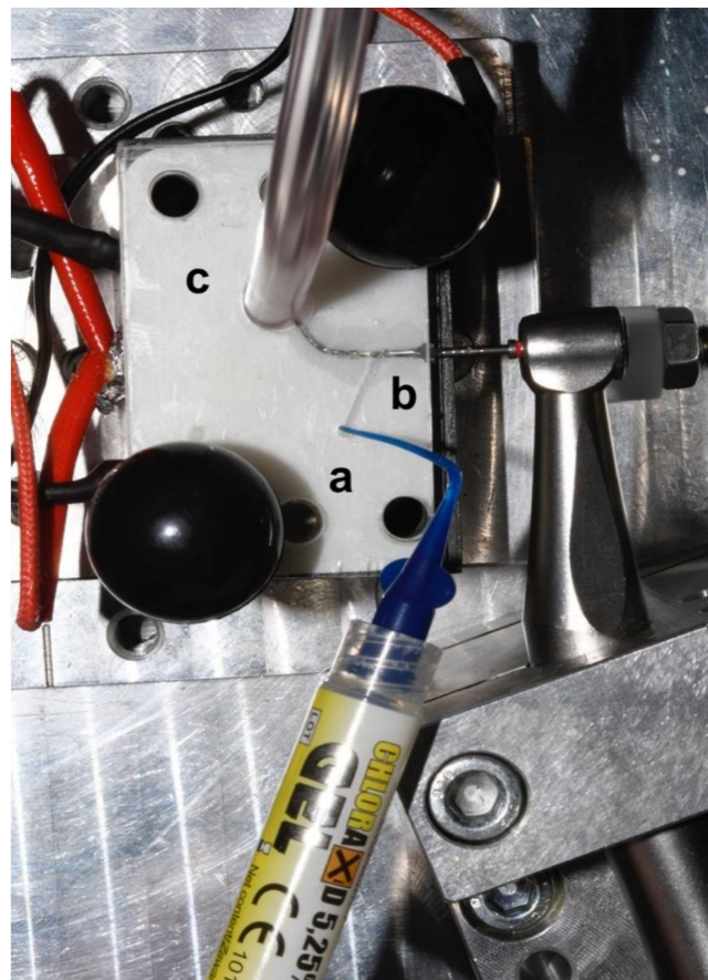
Figure 2. A detail of device with a F6 SkyTaper (F6ST) instrument exposed to NaOCl gel. (a) Irrigant tip insertion; (b) channel made inside the cover; (c) aspiration system allocated near to the canal apex.
