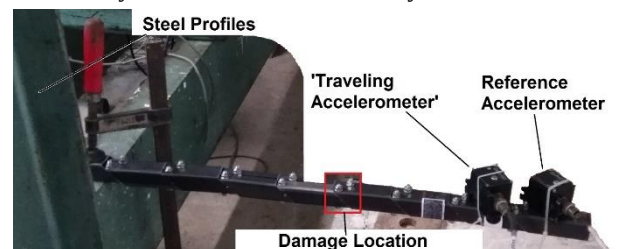
Figure 14. Experimental setup and the red box marks the damage position.
