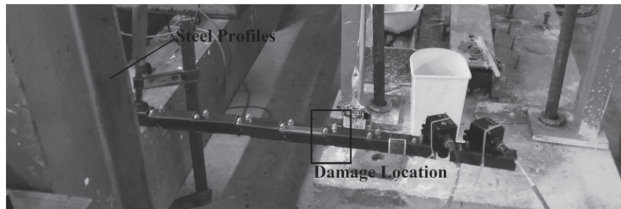
FIGURE 13 Experimental setup and black box showing damage position
